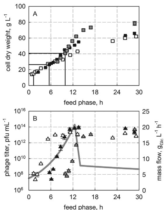
**Figure 3.** Cell dry weight and phage titer as function of time of infection. Fed-batch phage fermentations were carried out with infection at a cell dry weight of  $15 \text{ g L}^{-1}$  (white symbols),  $26 \text{ g L}^{-1}$  (black symbols), and  $40 \text{ g L}^{-1}$  (gray symbols). The cell dry weights (A), the phage titers and the glucose mass flow (B) are shown.
